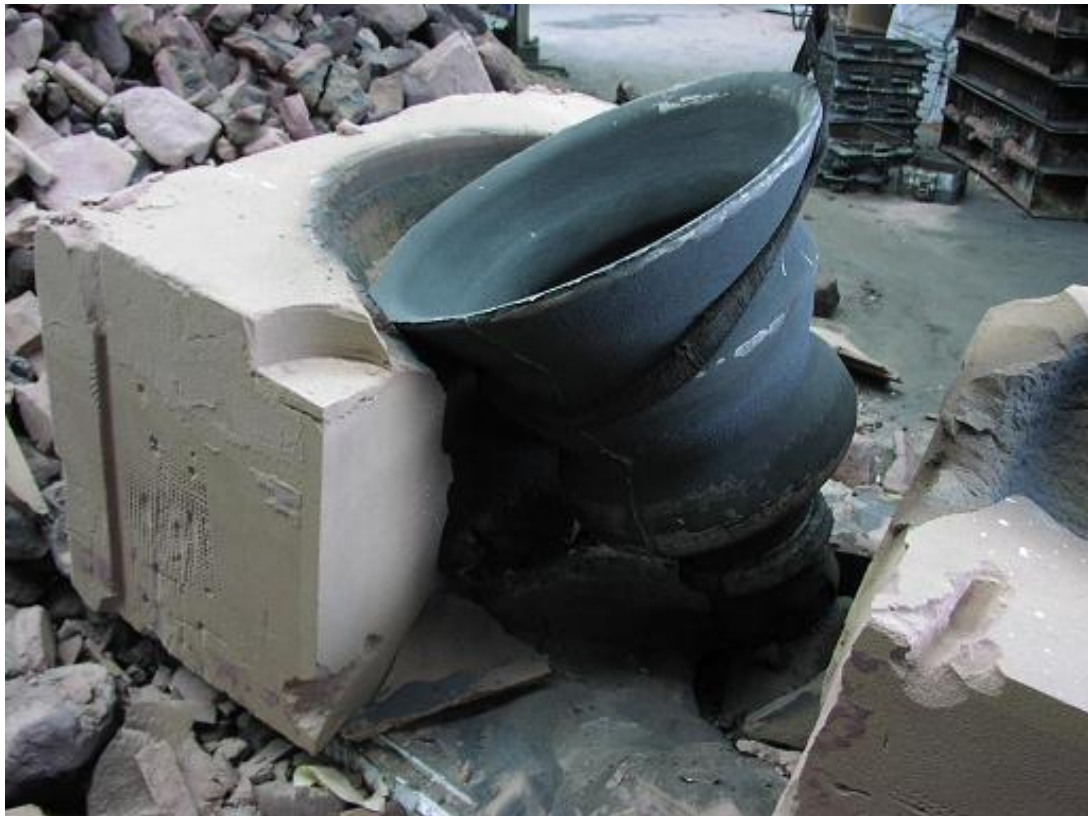
Fig1. One half of a Time and Tide Bell being broken out of the mold.
